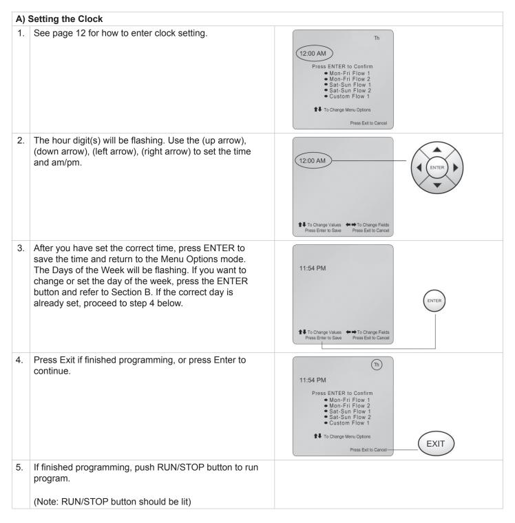
Please note: In the PROGRAM menu, if no button is pressed within 30 seconds, the unit will EXIT and return to the RUN mode.
