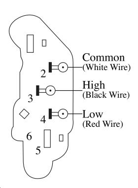
This two speed pump requires 3 line connections plus a ground wire. The typical color for wires from spa to motor are as follows:
