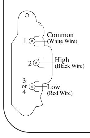
This two speed pump requires 3 line connections plus a ground wire. The typical color for wires from spa to motor are as follows:
