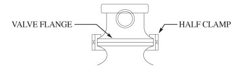
7. The plastic clamp can now be installed. Place clamp half over the valve flange and the tank flange as shown above. Insert the valve screws and nuts into the clamp half making sure that the nuts are located in the special hexagonal retainer slots on the clamps. See below.
