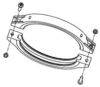
8. Tighten clamp screws firmly and visually check the valve tank and clamp assembly to insure that the joint is correctly assembled.
